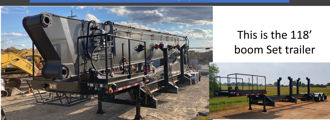
The trailer was designed to load the boom to the base machine over the goose neck keeping the overall length to 53'
