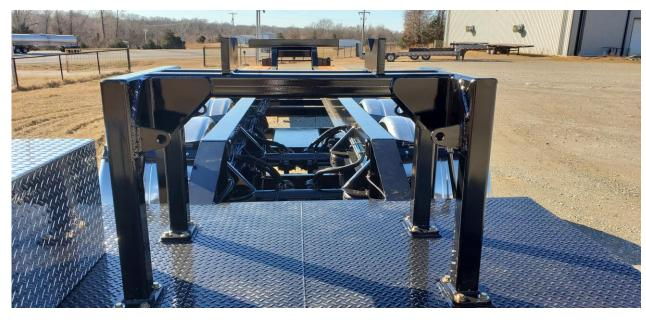
Equipped with lockable toolbox for chains binders and boom mounting equipment.
