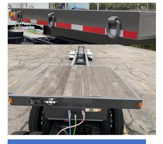
Goose neck area made for carrying tools 3 D rings per side
